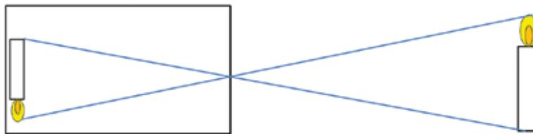
If the pinhole were enlarged, the image would get brighter, but less sharp. The bigger hole allows more light rays to pass through and illuminate different points on the screen, making the image appear blurry.
